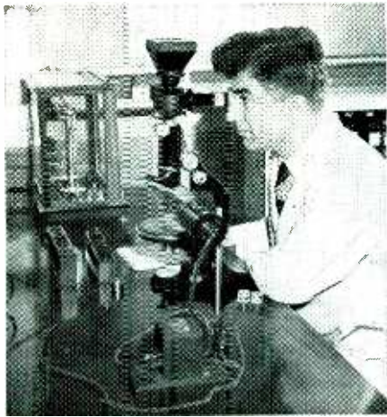
TO INSURE HIGH METAL QUALITY, Frank DePaola, chemist, studies samples microscopically for grain and crystal structure.
