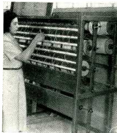
Simple rack holds up to 100 large spools of wire and provides convenient access to ends of wires
