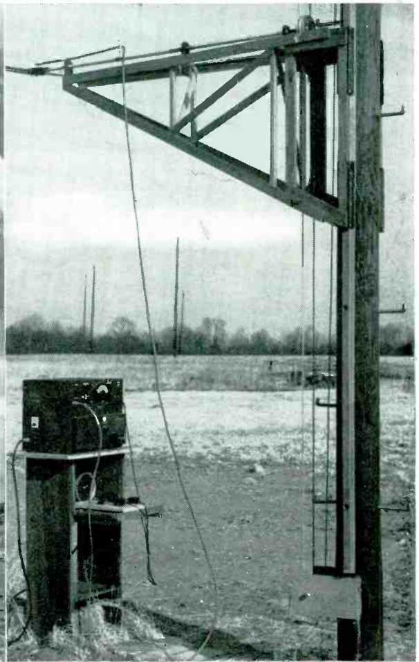
Field intensity meter uses antenna mounted so that antenna elevation and polarization can be changed by manipulating ropes
