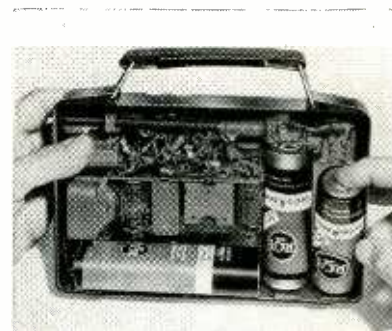
Rear view of the new RCA personal portable, showing the new alkaline B battery at the left
