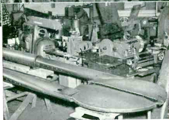
Photo taken in the University of Washington shop during fabrication of the two Ds and D Stems.
