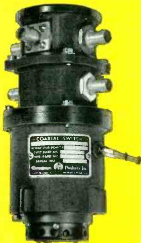
Model CA-31, 2P2T Sensing or Lobing Switch, 115 volt, 380-1000 cycle AC motor actuator. Switching speed, 15-35 Rev/sec. For use with RG-58/U cable.
