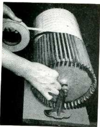
Winding adhesive tape spirally on drum made from removable U-channels, for cutting into tabs at Keystone Products Co.
